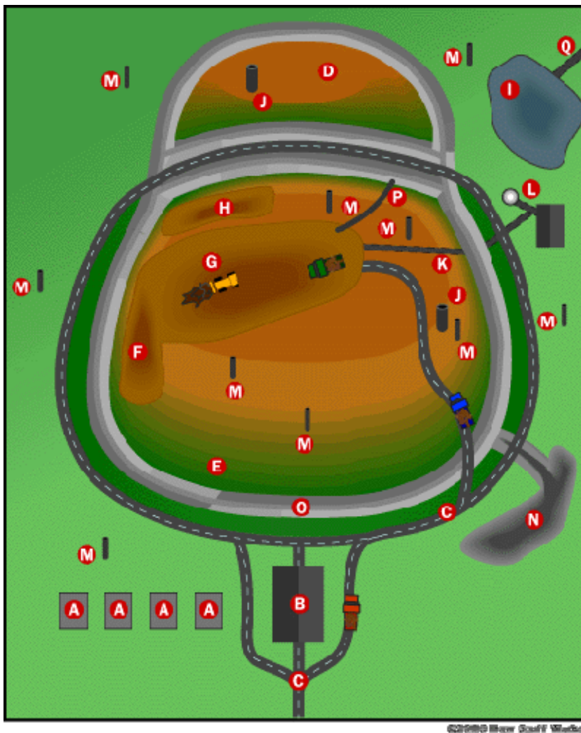
Figure 4. This overview shows the supporting stations and structures of a landfill. The drawing is based on the structure of the North Wake County Landfill in Raleigh, North Carolina.
